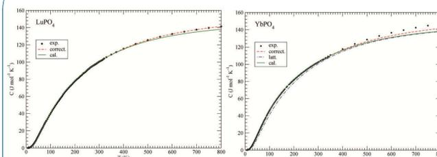
Fig. 6. The calculated and measured heat capacity of  $LuPO_4$  and  $YbPO_4$  [4].
