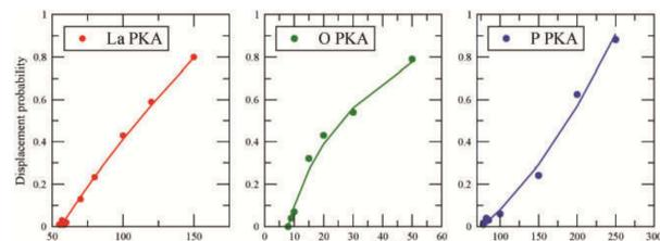
Fig. 2. The simulated atomic displacement probabilities of La, P, O PKA in  $LaPO_4$  at  $T=300K$  [1]
