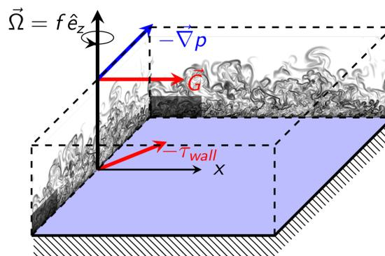
Sketch of the Ekman layer that develops from the interaction between a flow in geostrophic balance  $2\Omega k \times G\mathbf{i} = -\nabla p$  with the no-slip condition  $u = 0$  at the boundary  $z = 0$ . Stable stratification is imposed by a negative surface buoyancy  $B_{\text{wall}} = -B_{\text{ref}}$ .
