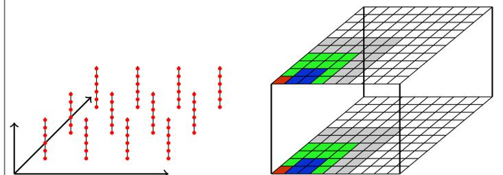
Illustration of the data employed in the convergence study. Left: individual towers distributed on a regular grid subsampling the flow in space. Right: coarse-graining procedure for a two-dimensional horizontal convergence (1D along the streamwise and spanwise directions is not shown)
