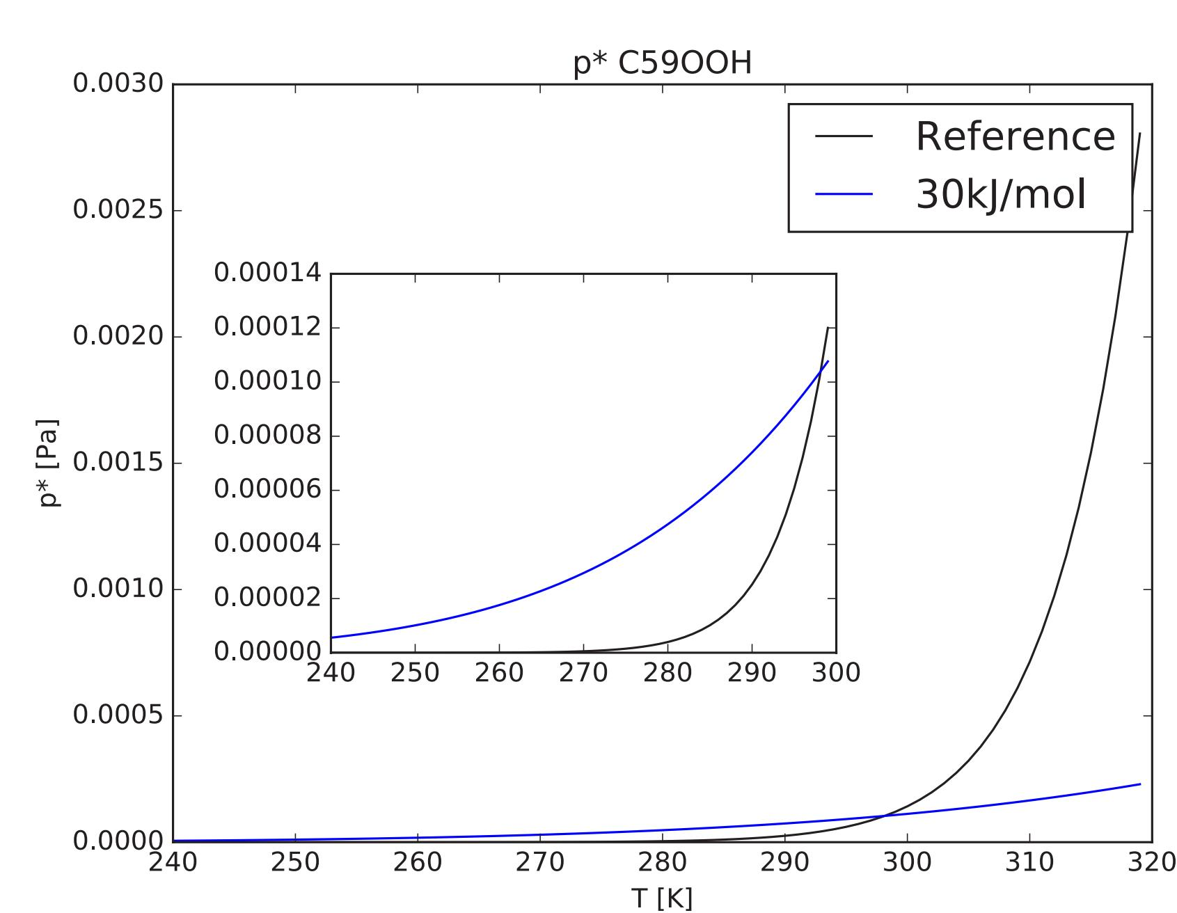
$$C_i^* = C_i^*(T_0) \frac{T_0}{T} \exp \left[ \frac{\Delta H_{\text{vap}}}{R} \left( \frac{1}{T_0} - \frac{1}{T} \right) \right]$$
