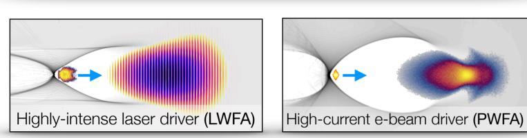
Laser and beam driven plasma wakefield accelerators
