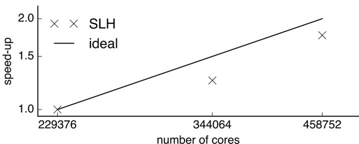
**Above:** Full-machine tests on JUQUEEN during the 2016 Extreme Scaling Workshop. The runs computed the Taylor-Green vortex on a  $2688^3$  grid with 16 MPI tasks per node and 4 threads per task.
