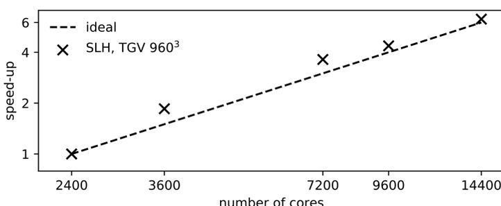
**Above:** Scaling test using the Taylor-Green vortex computed on a  $960^3$  grid with pure MPI parallelization on JUWELS.
