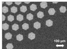
Optical microscope image of growing graphene flakes on liquid Cu at 1370 K. M. Jankowski et al., in preparation
