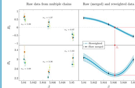
(a)  $B_3(|L|)$  and  $B_4(|L|)$  of different Markov chains (left) and of merged raw and reweighted data (right) (Wilson fermions,  $\kappa = 0.11$ ,  $N_\tau \times N_\sigma^3 = 6 \times 36^3$ )
