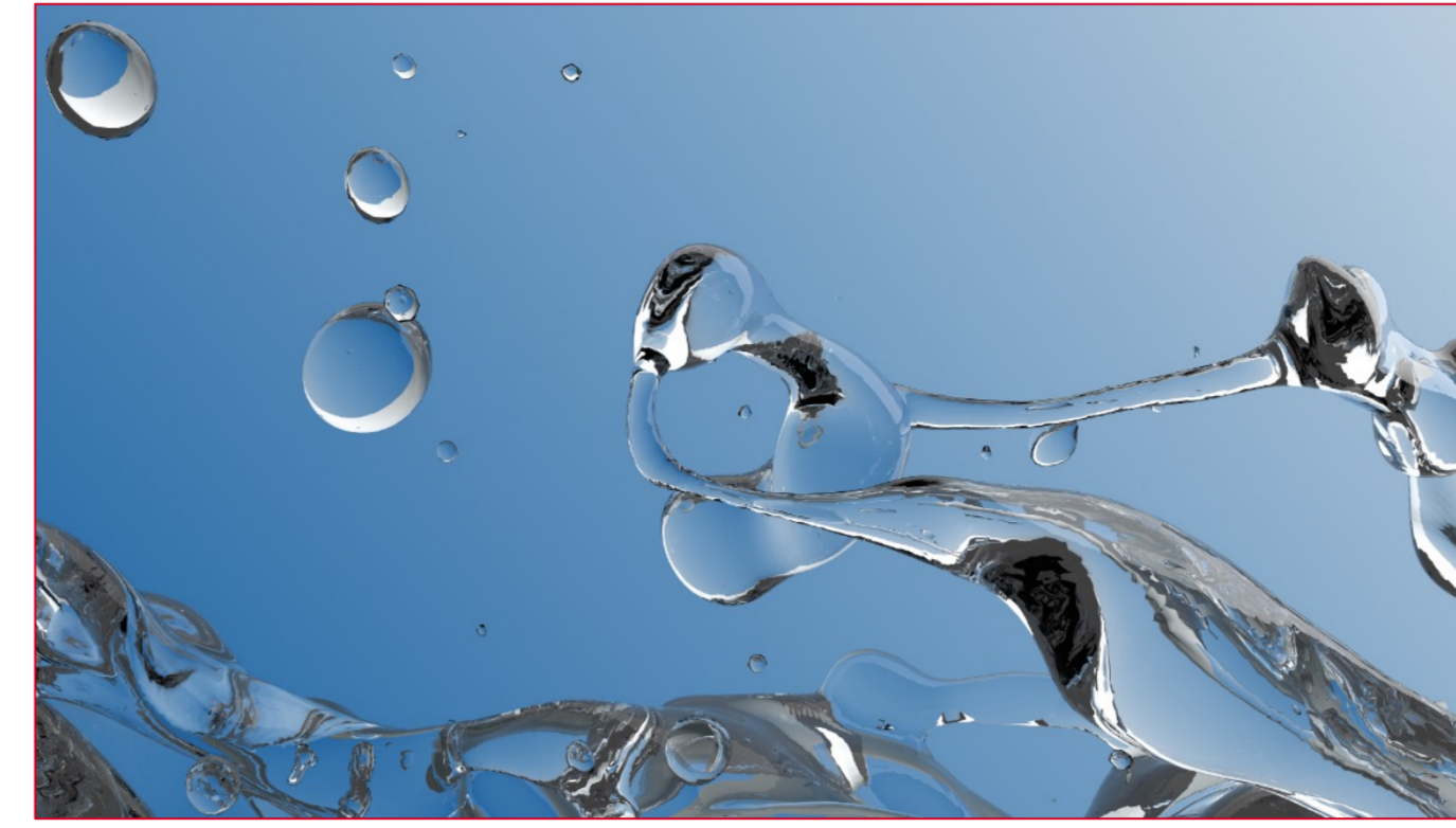
Fig. 1: Visualization of breakup DNS data (left) and complex engine LES (right). The highly-resolved DNS data can be used to train a data-driven subfilter model, which is then used to accurately model fuel injection in the LES.
